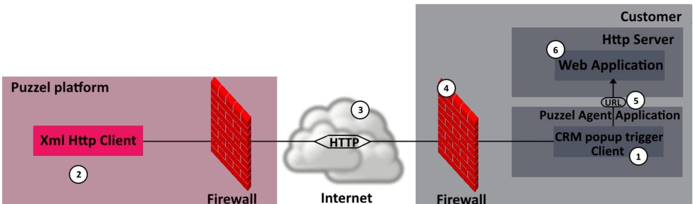
1. When the agent logs in using the Agent Application, contact is established with the trigger server on port 80 using HTTP. The contact is kept open as long as the agent is logged on to Puzzel and the Agent Application is running.
