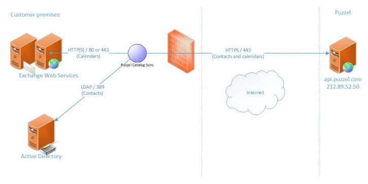
The diagram above shows connectivity in an environment where Exchange is installed on premise. For Office 365 the Exchange server will be in the cloud but it is the same kind of communication and over the same ports.
