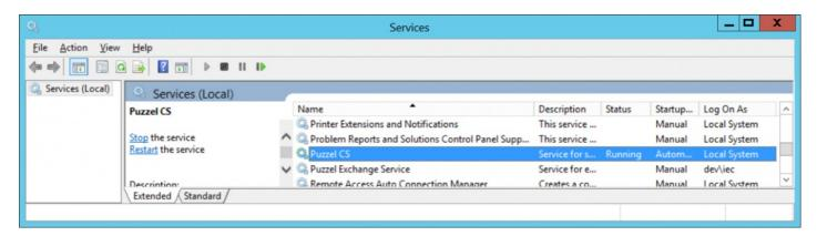
Verify that the service is running in context of the correct user. This is the service account that have been created and configured earlier. If this is not the account entered in the "log on" tab, enter it now. Note that this is only necessary if integrated authentication was chosen in the configuration tool. If "specify user and password" was chosen those credentials will be used instead.
